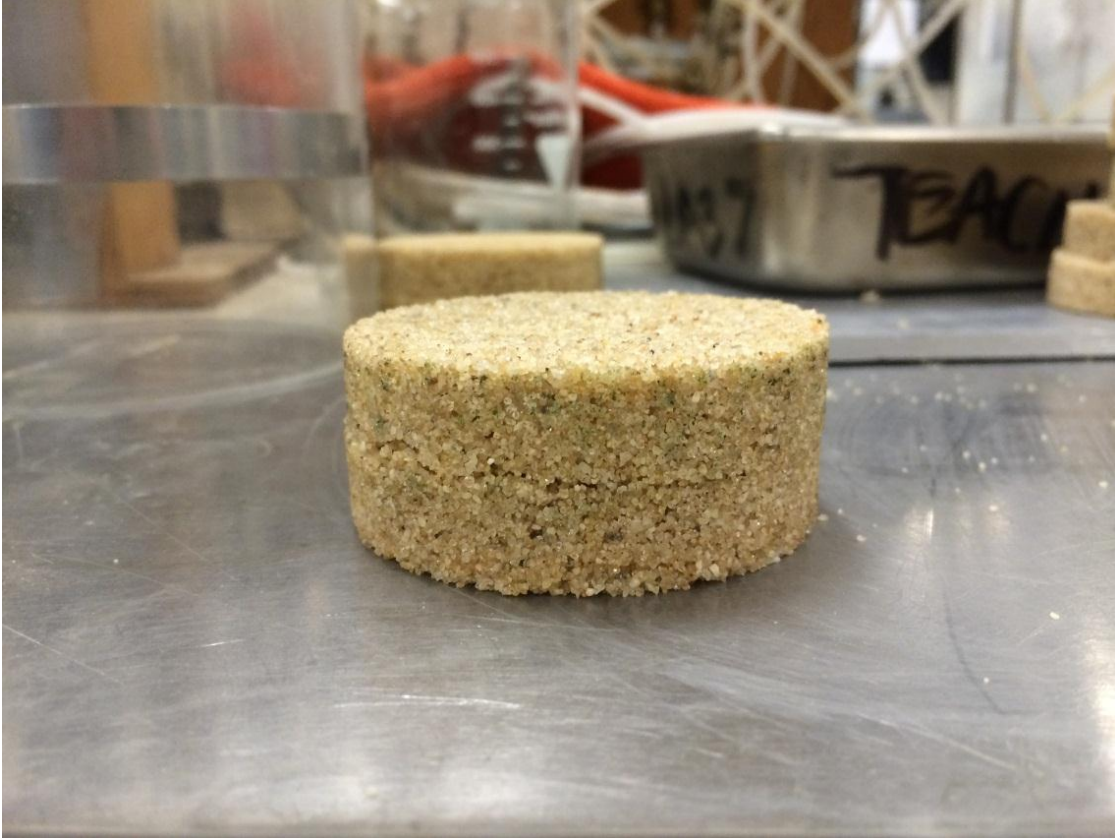
Figure 75. Healed 4% polymer-amended sand specimen 7 days after first DS test.
