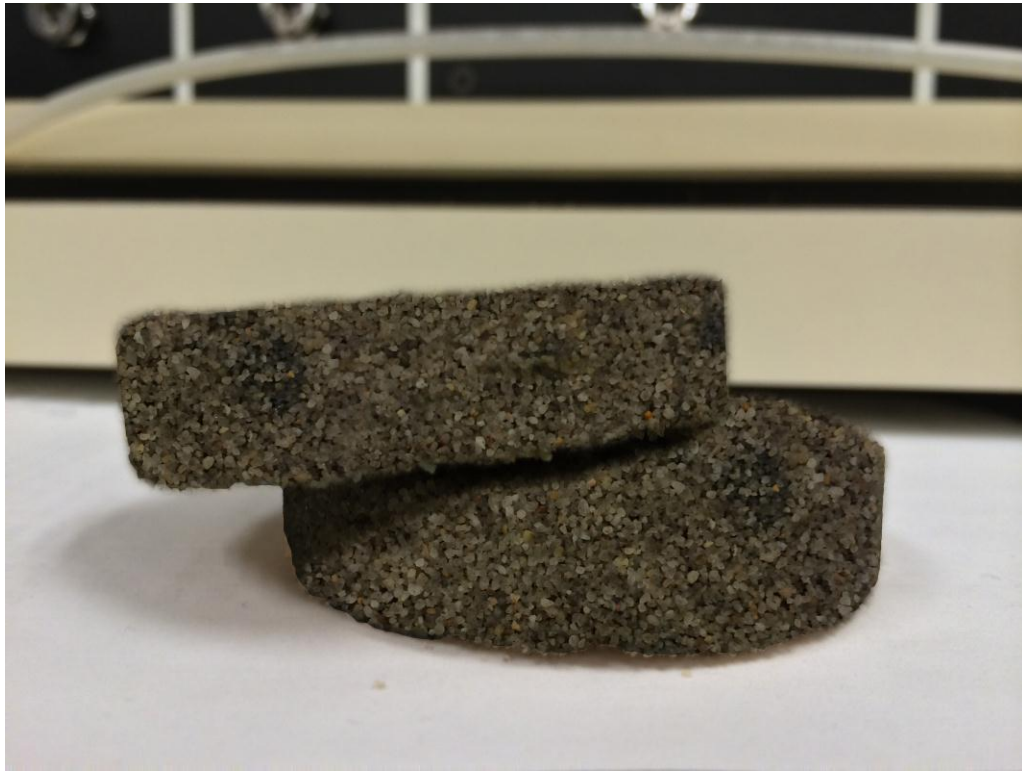
Figure 32. 8% cement-amended sand specimen after failure.
